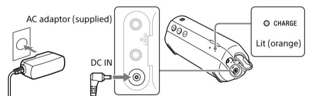
Charging starts when the unit is connected to an AC outlet via the AC adaptor, and the CHARGE indicator (orange) lights up. Charging is completed in about 3 hours and the indicator goes off.
